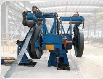
Double Mandrel Rotatable Uncoiler for tube sizes of < \phi 89\text{mm}
